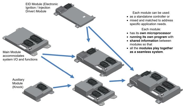
Each of the basic LECM platform modules has its own dedicated complement of inputs and outputs as shown below.
